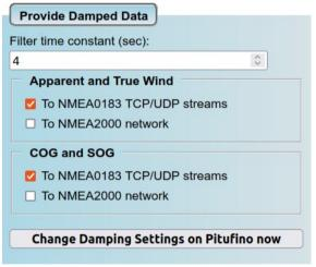
apps/displays should then be disabled). If your apps/displays do offer adequate damping but you wish to use the true wind computed by Pitufino, 'Apparent and True Wind' need to be enabled in Pitufino's settings, but the filter time constant should be set to 0 seconds. Note, Pitufino's browser-
