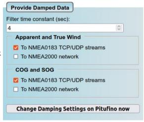
COG/SOG in your apps/displays should then be disabled. If your apps/displays do offer adequate damping but you wish to use the true wind computed by Pitufino, 'Apparent and True Wind' need to be enabled in Pitufino's settings, but the filter time constant should be set to 0 seconds. Note,
