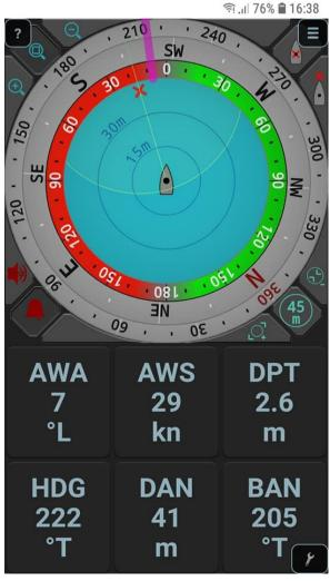
Pitufino keeps track of how many turns (i.e., rotations or 360s) your vessel does while at anchor. For instance, @ 2.5 means it turned clockwise two and a half times. In some anchorages (i.e., changing currents, wind against current, or catabatic winds from different directions) this info can be useful for untwisting your chain again. Pressing this button resets the counter.
